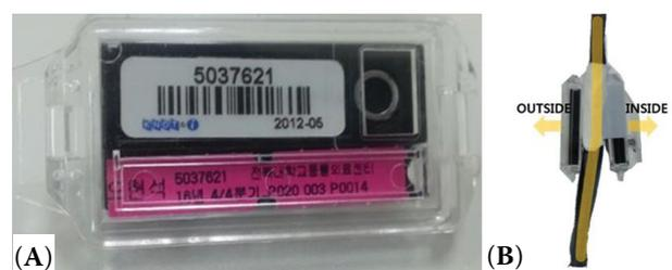
Figure 2. (A) shows a TLD used in this study for measuring the cumulative equivalent dose, and (B) shows how TLDs were attached inside and outside of the lead apron
