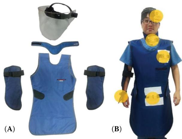
Figure 1. Picture (A) shows the lead protective devices, which were a lead mask, thyroid shield, apron and hand shield. Picture (B) shows the locations where the TLDs were fixed on the body
